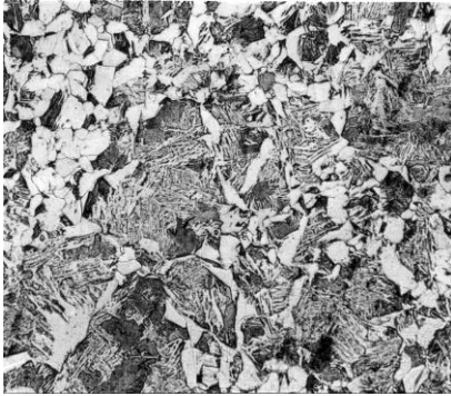
Figure 6 – Microstructure of the core area in 6.0 - mm-diameter reinforcing wire of referenced micro-alloyed by B low - carbon steel; TMCR schedule 3.1 with T_{LH} = 920^\circ C ; magnification 800X.
