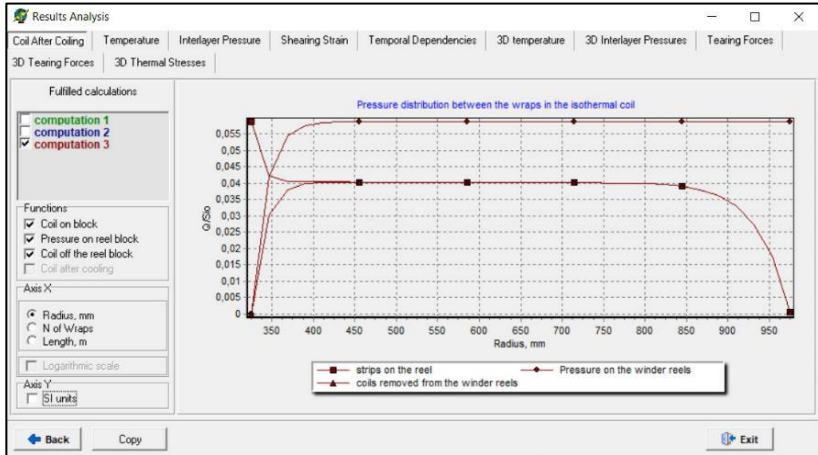
Figure 4 – Distribution of inter-turn pressures in the roll.
